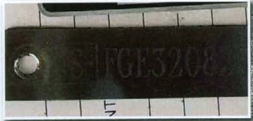
A fraudulent outdrive serial number found on the Volvo-Penta outdrive of a stolen Cobalt.
