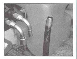
gine for damage. Volvo added an additional two years of extended warranty to both engines. At 47 hrs same hose again came off barbed nipple.
