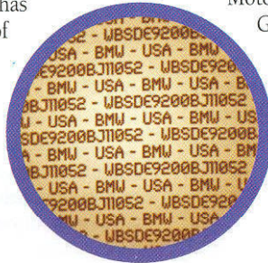
Painting a hull with invisible Data Dots IDs a boat under UV light.
